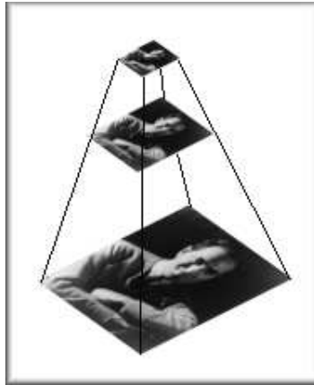
Figure A.1: A multi-resolution approach illustrated. Coarser representations are shown at the top levels and the original image lies at the bottom.
